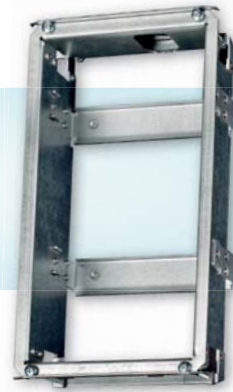
Plasterboard mount box Dimension: 237 x 129 x 70 mm Hole: 237 x 118 mm (Ord. num. 9151002)
